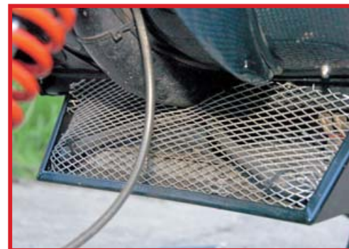
Mesh has added to give extra radiator protection
