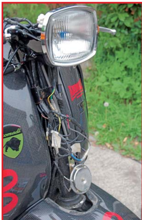
Soldered at both ends, changing a broken throttle cable can be a bit of a task!
